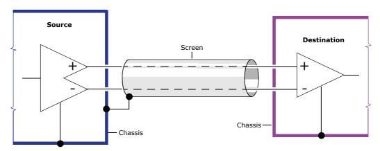
Screen termination diagram showing screen broken at destination
