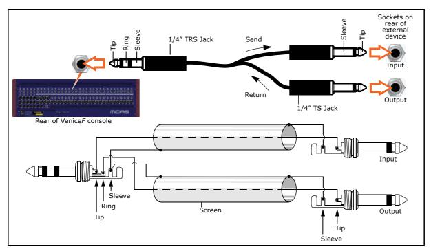
Figure 2: Connecting to unbalanced equipment
