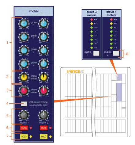
matrix output section on the control surface
