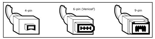
Figure 3: Some typical FireWire connectors
