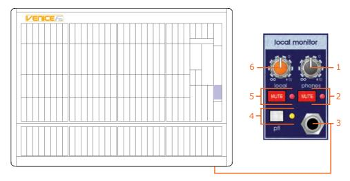
Local monitor section on the control surface and the position of the addition headphones socket on the front panel of the console
