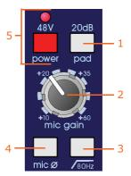
Mic gain section of the mono input channels
