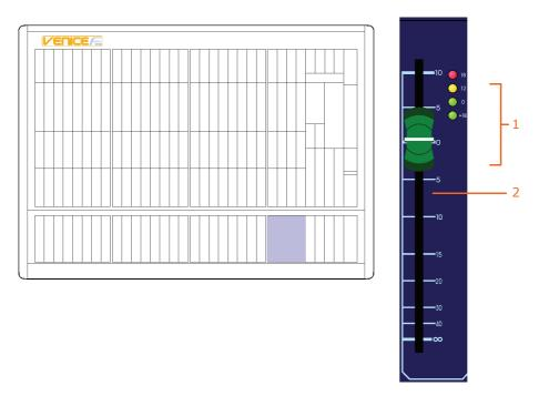
Fader section of the dual stereo input channels
