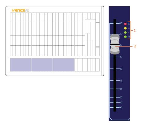
Fader section of the mono input channels
