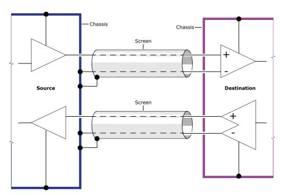
Ground referenced insert wiring diagram. For a typical example of how to wire a ground referenced insert, see Figure 1 on page 14; the example above shows the screen connection at the other end because it is more practical, as it reduces the wiring complexity within the 1/4" TRS Jack connector.
