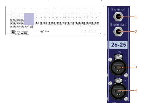
Dual stereo input channel connectors
