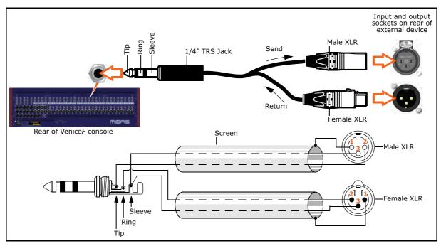
Figure 1: Connecting to balanced equipment
