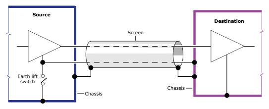
Ground lift connection on source
